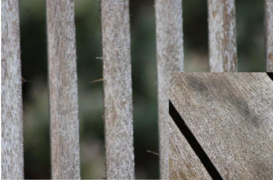
Power washers are very effective at blasting off dirt and old coatings but they also create furring and splinters on the timber.
